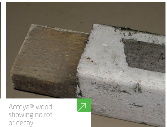
Non-acetylated wood showing severe rot and decay
