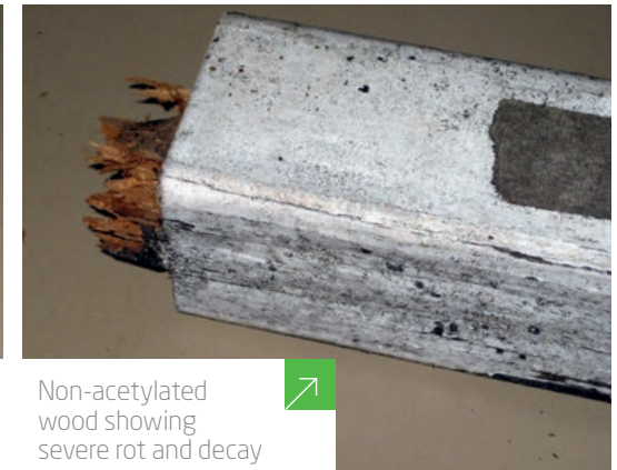
Non-acetylated wood showing rot and decay
