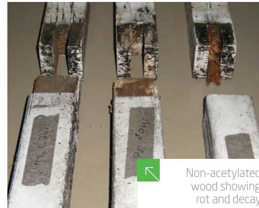
Non-acetylated wood showing severe rot and decay
